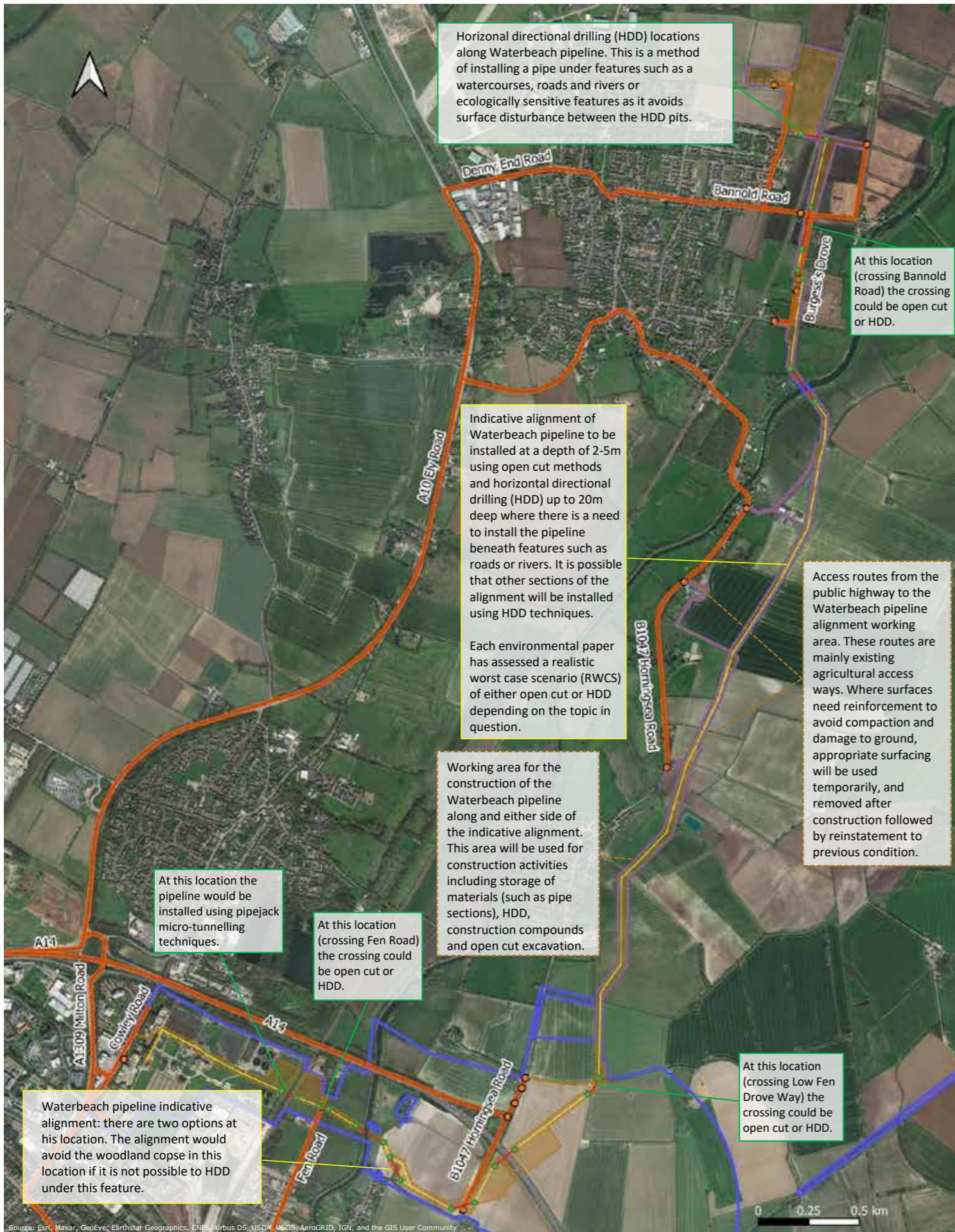
Cambridge Waste Water Treatment Plant Relocation Project – Preliminary Environmental Information Working Areas During Construction – Waterbeach Pipeline Route Legend Draft Scheme Order Limits Construction traffic routes (HGV) Construction traffic vehicular access point Waterbeach pipeline working area Pipeline installed using open cut methods HDD pipeline install below ground, unless otherwise stated
